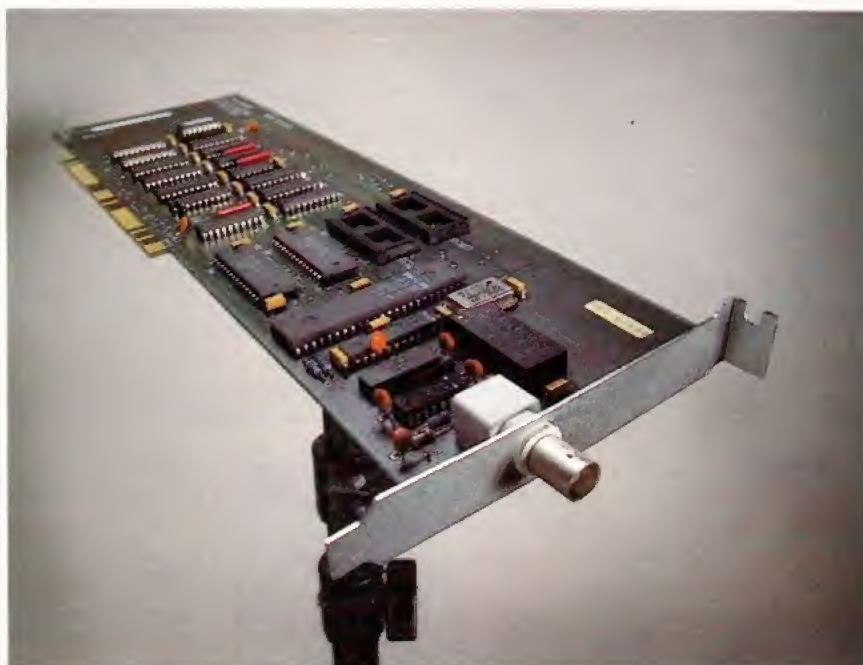
Ethernet cards are available for big-box Amigas, but why can't some cheaper, simpler network interface be included with the new Amiga as standard?
